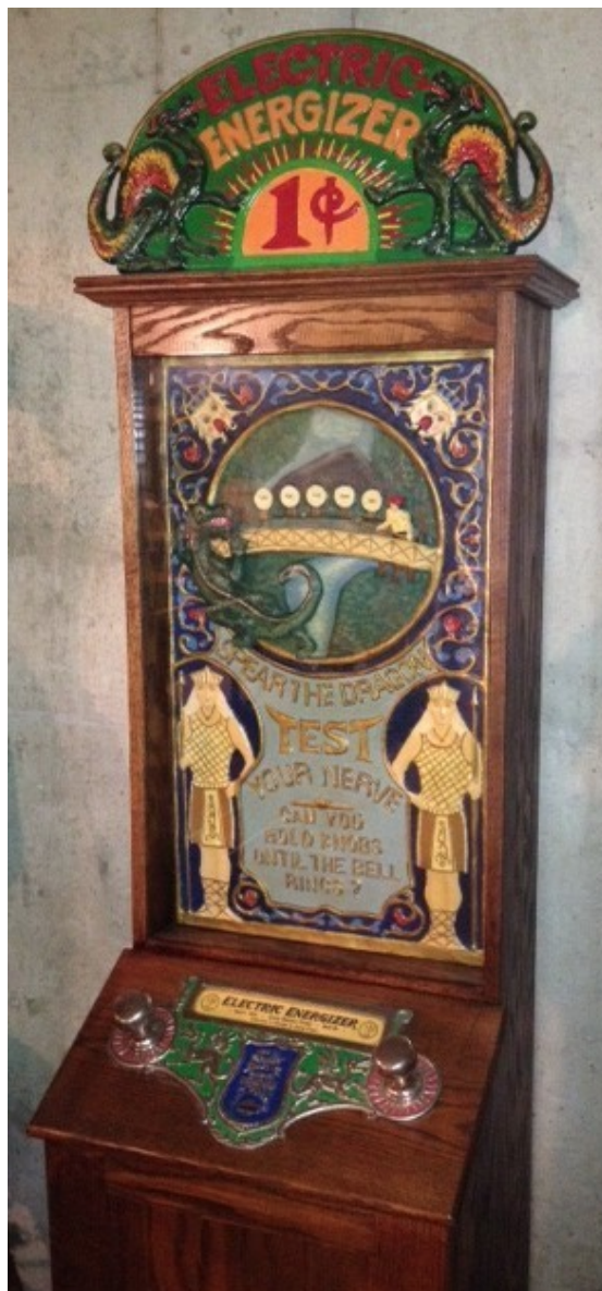
Figure 4: Spear the Dragon (1927) required the player to hold metal handles and withstand gradually-increasing shocks as the avatar moved toward the fire-breathing dragon.
